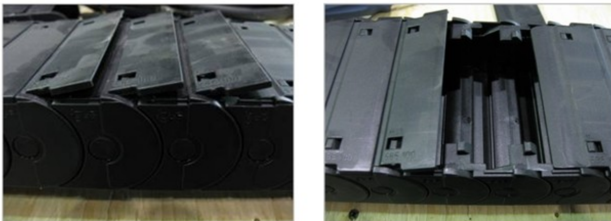
Figure 2 – RTW 3.0 Damaged Cover (2 of 7)
