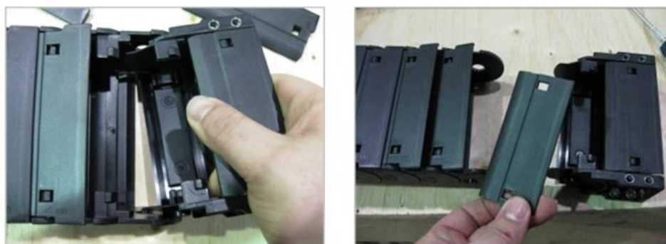
Figure 7 – RTW 3.0 Damaged Cover (7 of 7)
