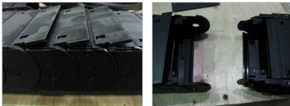
Figure 6 – RTW 3.0 Damaged Cover (6 of 7)
