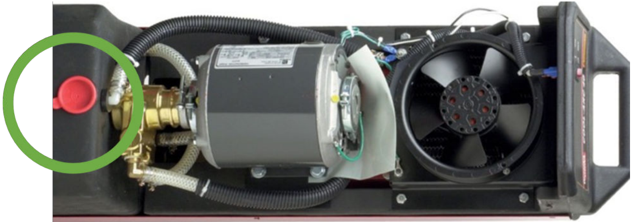
Figure 11 – RTW 3.0 Drain Coolant From The Pump Inlet Reservoir
