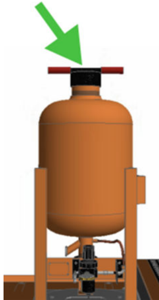
Figure 23 – RTW 3.0 Pressurized Flux Tank (1 of 3)
