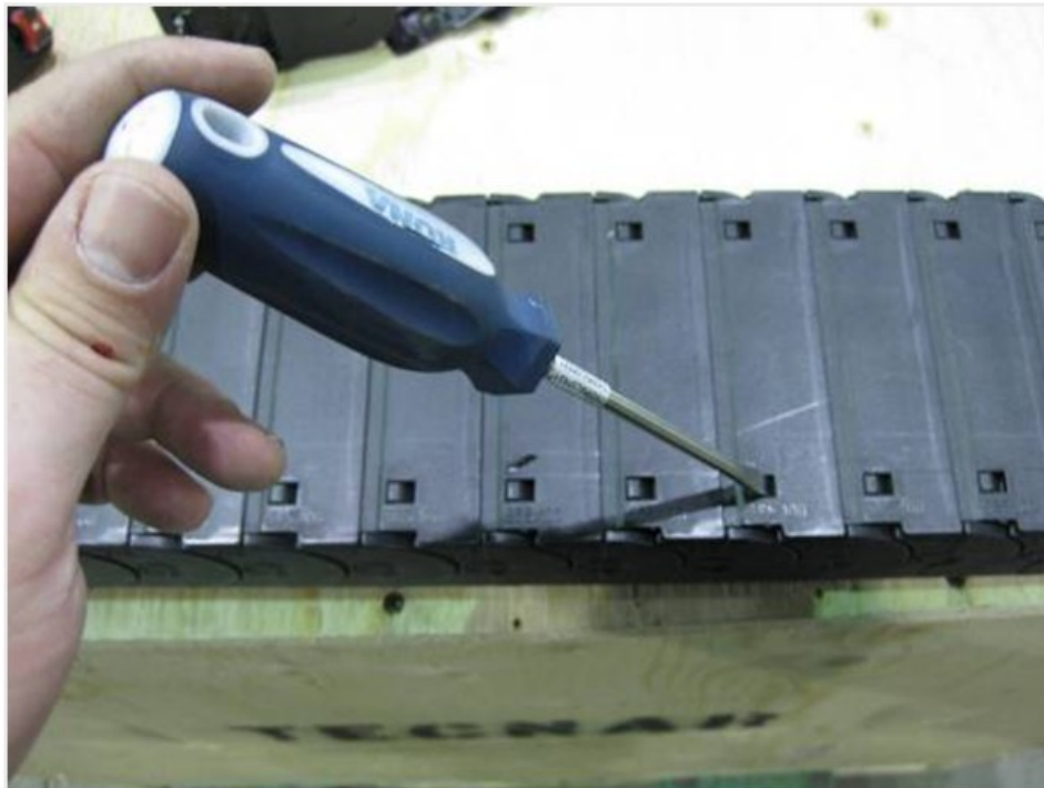
Figure 1 – RTW 3.0 Damaged Cover (1 of 7)
